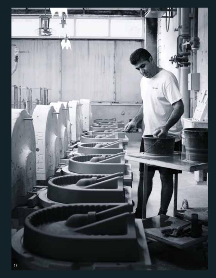
O1 Plaster molds are filled and stirred by hand; they have to be replaced by new ones after having been filled around 80 times.
